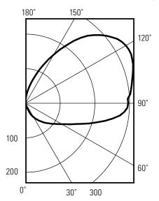
1050SQINFBW Report No. 3891FR Lamp: 4 Pin, 26W PLT, GX24q-3 Base Initial Lamp lumens: 1800 Luminaire Efficiency: 36.6%
